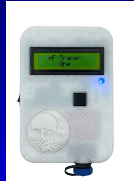
pF Tracer One by WETRUF for measuring the water potential or pF
